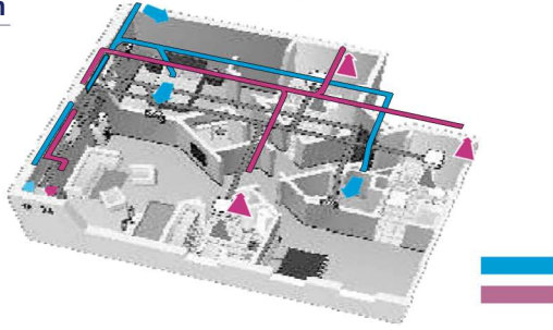
Fully Ducted System
