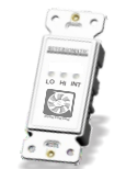
Intermittent Switch (IC 100-5V) Low/High/Intermittent/Off mode. In Intermittent mode, HRV/ERV runs for 20 min. in low speed & 40min. OFF. and cycles Continuously. (Also available w/o OFF mode)
