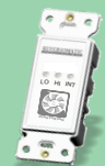
Intermittent Switch (IC 100-5V) Low/High/Intermittent/Off mode. In Intermittent mode, HRV/ERV runs for 20 min. in low speed & 40min. OFF. and cycles Continuously.
