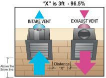
Double Vent (DVG-200) c/w extruded aluminum grilles Re - Circulation Efficiency - 95%
