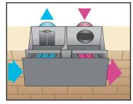
Double Vent (DVV-100C) c/w vertical Exhaust / Intake hood Re - Circulation Efficiency - 98%
