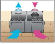
Double Vent (DVS-100) c/w side Exhaust / Intake hood Re - Circulation Efficiency - 98%
