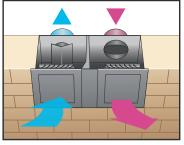
Double Vent (DVS-100) c/w side Exhaust / Intake hood Re - Circulation Efficiency - 98%
