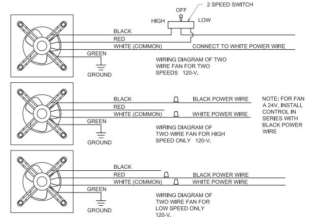
Note:- For A-30 & A-36 wiring diagram & rotation change see the motor name plate.
